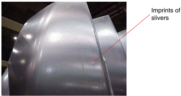
Fig. 1 Imprints of slivers into stamped panels
